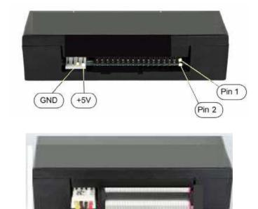
Connect the device as shown in the figure, the pin 1 of the flat is colored blue or red. The power of the device usually 4 wires, 5 V should be connected as shown.
